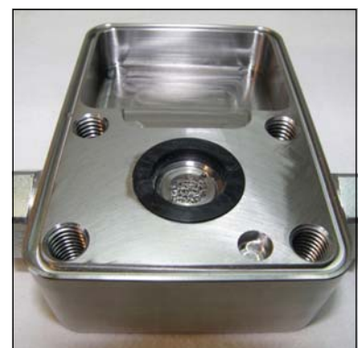
Fig. 3 - Bottom part sealing ring and sinter filter
