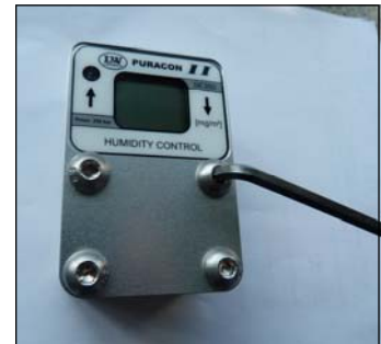
Fig.1 - Loosen cover screws, do not extract
