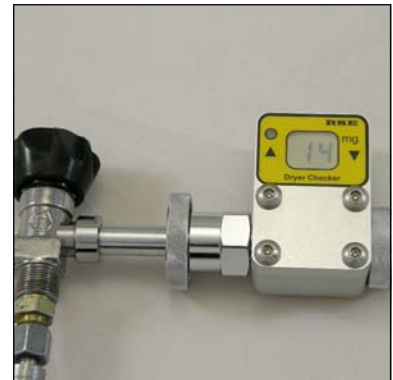
Connect Puracon Mobile to the compressor filling hose
